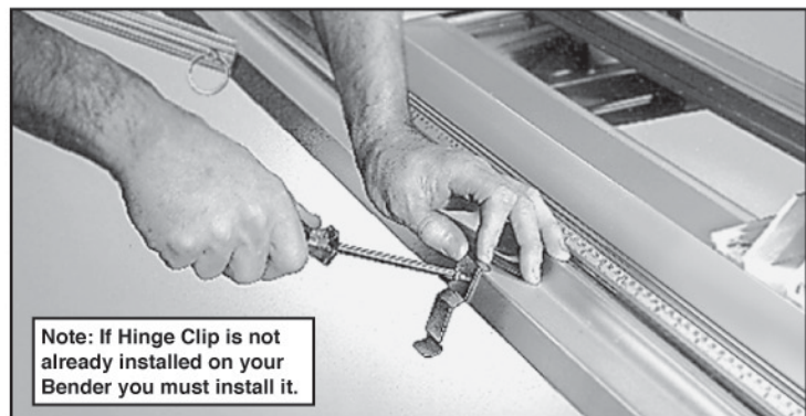
Figure 1. The Hinge Clip keeps the Moving Hinge in a 90° position for ease of aligning and cutting material. To install Hinge Clip, locate pre-drilled hole on BOTTOM right side of Moving Hinge. Align holes in Clip and Hinge as shown and insert Phillips head screw provided.
